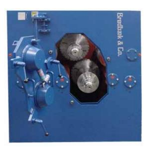
The new BCO 800/60 at work, producing up to 50 boards/min.
