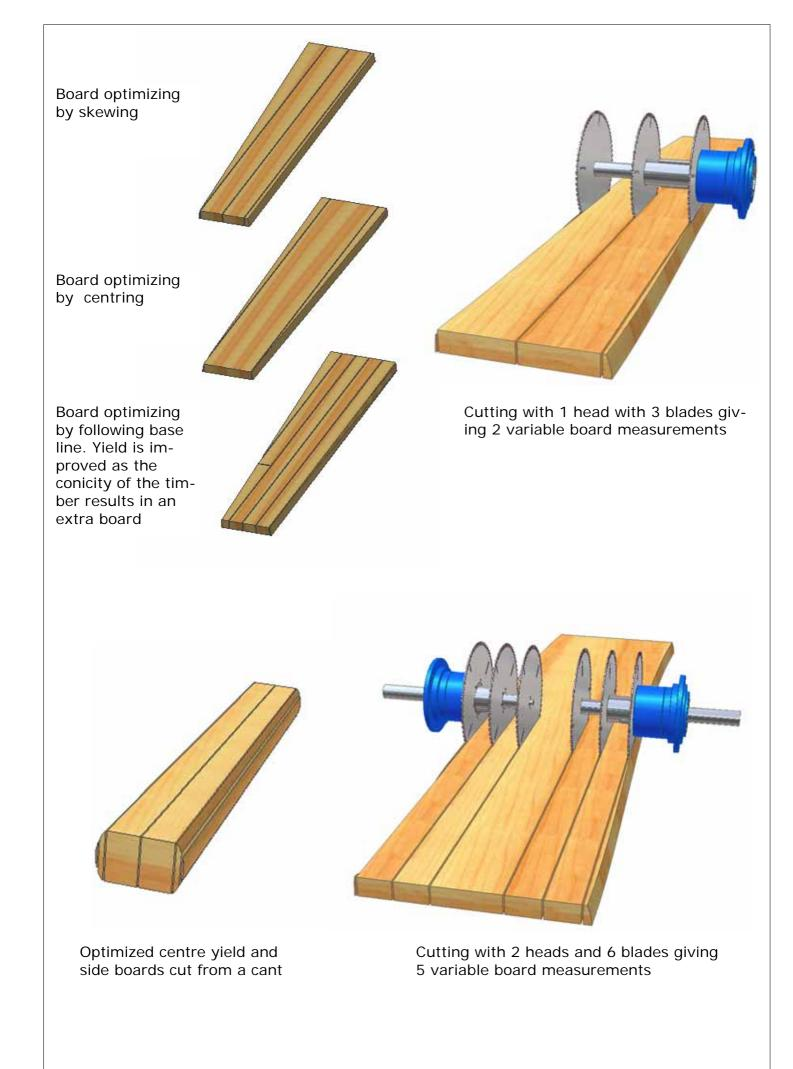
Below another modular built solution based on our indeed flexible circular saw. The BCO 800/180 circular saw is mainly used for cant sawing - here shown in combination with our chipper canter BCO 500. Equipped with ø650 mm saw blades the cutting depth will be 50 to180 mm, and feeding speed will be up to 150 m/min.
