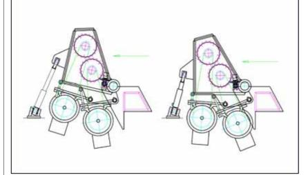
The vertical movement of the saw positions the saw blades correctly according to required cutting height. Upper and lower saw blades cut at the same depth. The saw changes vertical position to follow log taper
