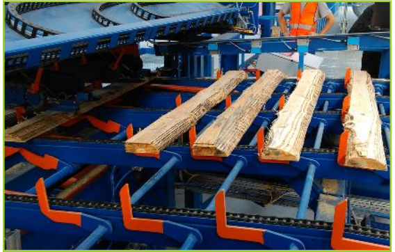
Bundles of 10 slats on Stelmet's special stacking machine.
